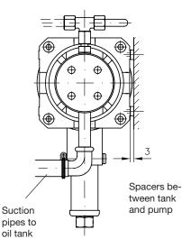
b) Pump mounted with cylinders turned by 90°
