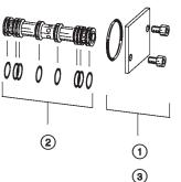
Push out the main plunger (any side) the sleeve remains in the housing. Lube the visible sections of the O-rings.
