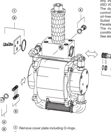
Any industrial standard hydraulic oil (ISO VG 10) or spindle oil (ISO VG 5 to 10) may be used in the pneumatic maintenance unit. The dynamic seals of piloting and main plunger of the reversal control valve should be lubed regularily when connected to oil-free pneumatics and frequent every-day use is intended. Suited are longterm lubes e.g. Autol TOP 2000 from Co. Autol, Paradiesstraße 14, D-97080 Würzburg.
