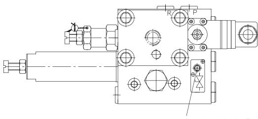
Accumulator drain valve a/f 5 1)
