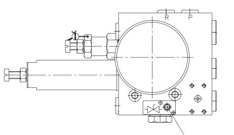
Accumulator drain valve a/f 5 1)
