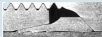
Cross section - Two-edge cutting ring
