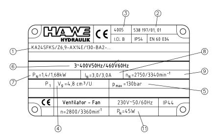
Type plate for hydraulic power pack with 1-phase motor
